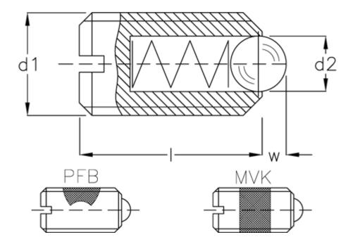
$\begin{array}{ll} d1 & = M10 \\ d2 & = 6.0 \\ Length I & = 19 \\ Spring pressure N bottom = 104.0 \\ Spring pressure N top & = 57 \\ W & = 2.0 \end{array}$
